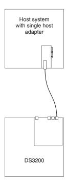
Figure 26. Single-controller direct-attached connection to a single-host HBA
